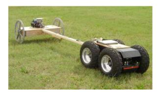
Fig. 2. Picture of Segway and Trailer
