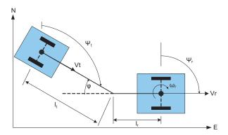
Fig. 3. Schematic Representation of Segway and Trailer
