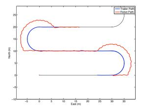
Fig. 8. Simulation Result: GPS on Robot &  $l_t = 6m$
