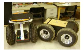
Fig. 1. Left: Segway RMP 200ATV Right: Segway RMP 400
