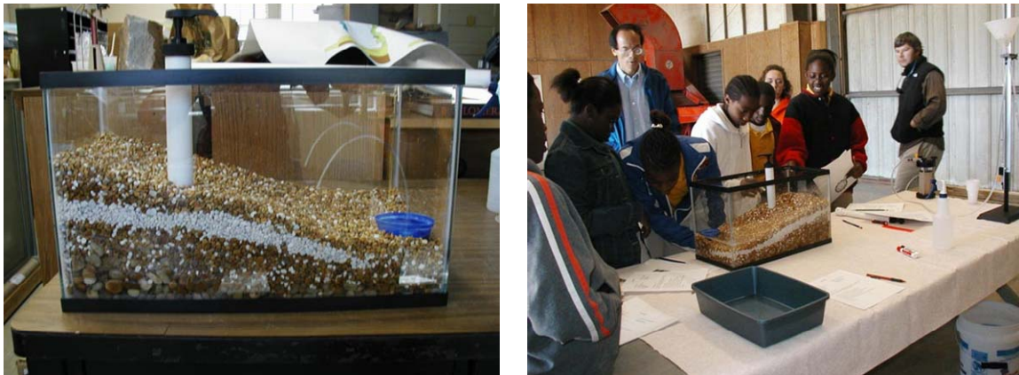
Figure 1. An aquifer tank model built to demonstrate groundwater and surface water interaction and groundwater contamination. Students can see and mark saturated zone, water table, unsaturated zone. They also examine the well casing and screen. They add water to simulate recharge, and pump water from well to simulate drought and overuse.
