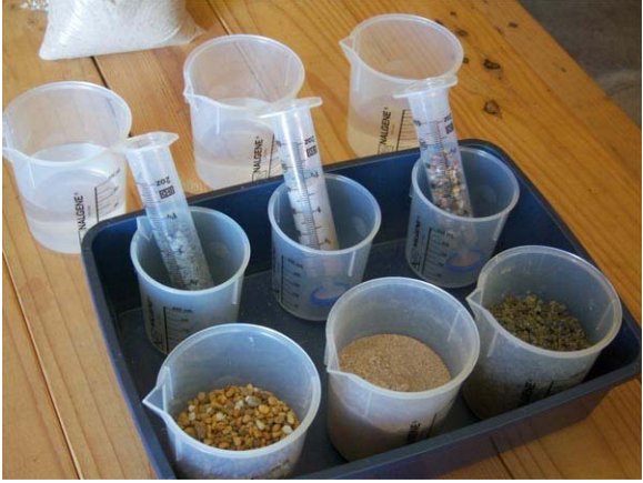
Figure 2. Students assemble “aquifer in a beaker” and “aquifer in a syringe” models to compare the porosity and permeability of gravel, sand, and clay-rich sediments.
