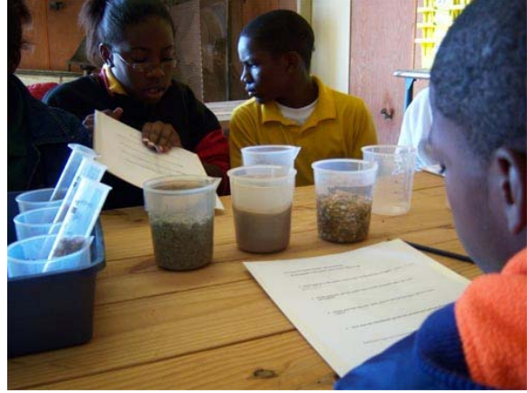
Figure 2. Students assemble “aquifer in a beaker” and “aquifer in a syringe” models to compare the porosity and permeability of gravel, sand, and clay-rich sediments.
